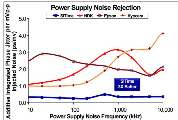
Figure 4. Power Supply Noise Rejection<sup>[4]</sup>
