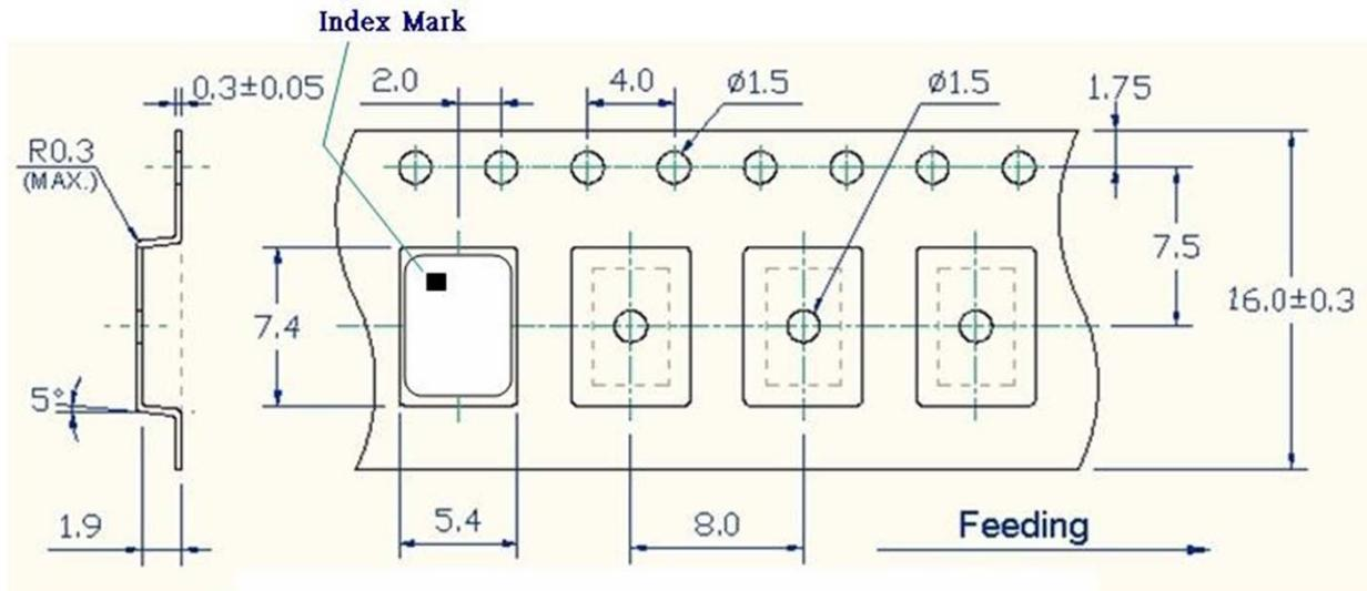
1. 230mm minimum leafer which consist of carrier and/or tape followed by a minimum of 160mm of empty carrier tape sealed with cover tape.
