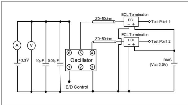
Fig.1 Test Circuits
