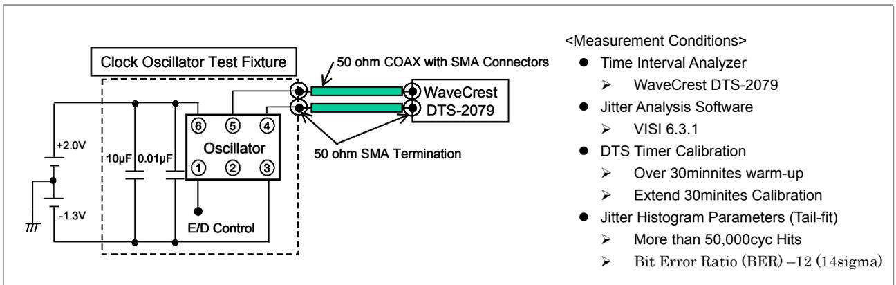
Fig.3 Jitter Test Circuits
