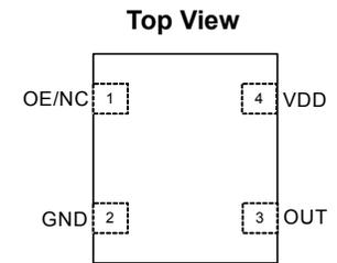
**Figure 1. Pin Assignments**
