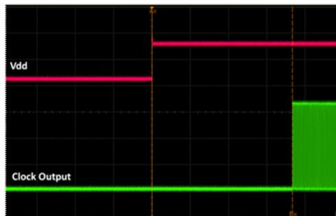
**Figure 16. Startup Waveform vs. Vdd**
