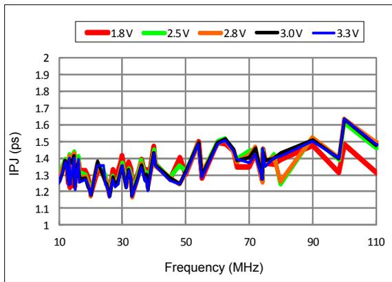
**Figure 13. RMS Integrated Phase Jitter Random (12 kHz to 20 MHz) vs Frequency<sup>[11]</sup>**
