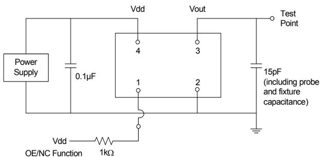
Figure 2. Test Circuit
