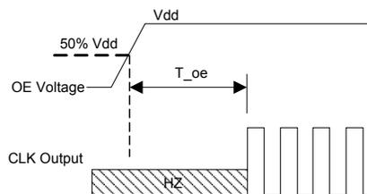
T\_oe: Time to re-enable the clock output
