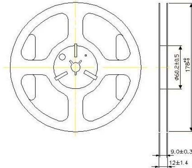
1. 230mm minimum leader which consist of carrier and/or tape followed by a minimum of 160mm of empty carrier tape sealed with cover tape.
