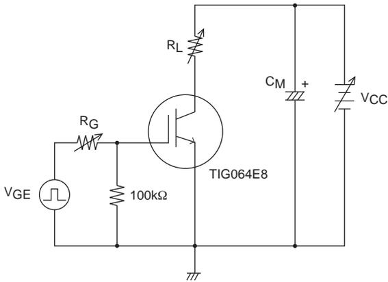
Note1. Gate Series Resistance  $R_G \geq 160\Omega$  is recommended for protection purpose at the time of turn OFF. However, if  $dv/dt \leq 400V/\mu s$  is satisfied at customer's actual set evaluation,  $R_G < 160\Omega$  can also be used.
