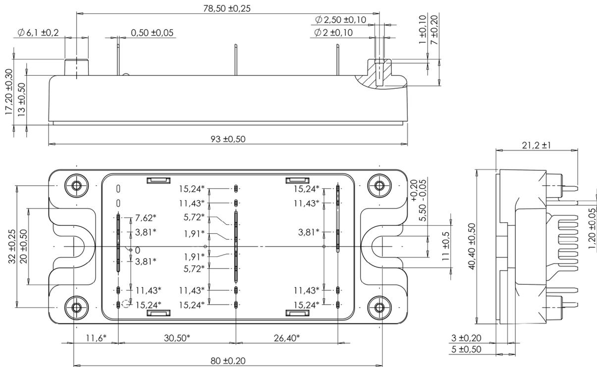
ALL DIMENSIONS MARKED "\*" ARE TOLERANCED AS:  $\pm \phi 1$
