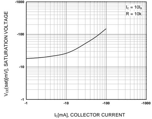
Figure 2. Collector-Emitter Saturation
