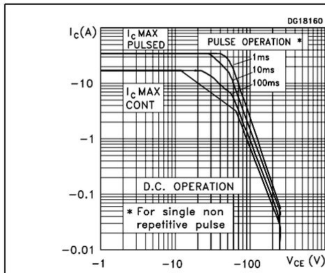
Figure 3. Derating curve
