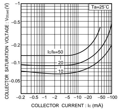
Fig.6 Collector-emitter saturation voltage vs. collector current (I)
