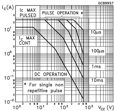
Figure 4: Derating Curve
