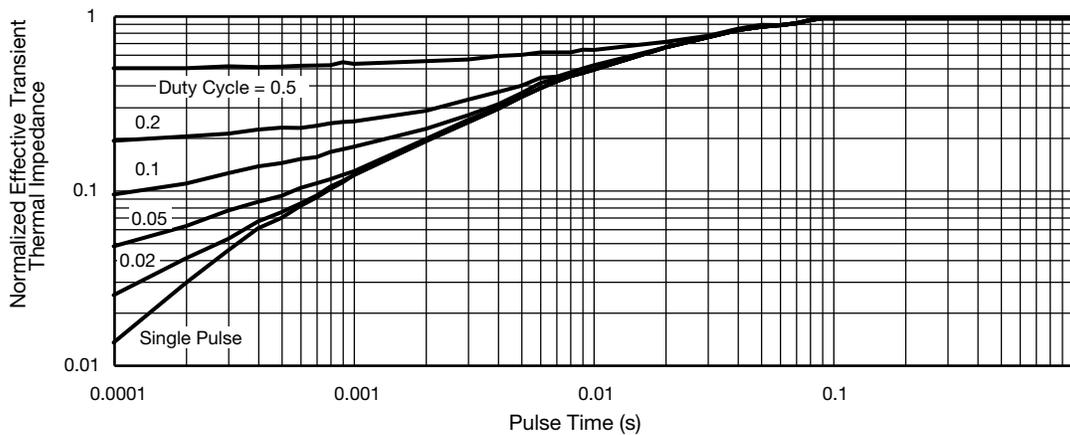
Fig. 11 - Normalized Thermal Transient Impedance, Junction-to-Case
