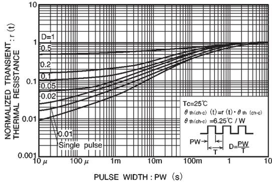
Fig.15 Normalized transient thermal resistance vs. pulse width
