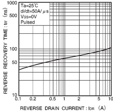
Fig.14 Reverse recovery time vs. reverse drain current
