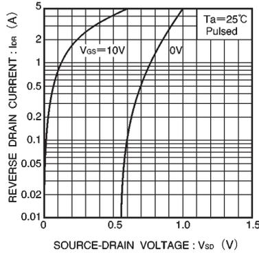
Fig.11 Reverse drain current vs. source-drain voltage (II)
