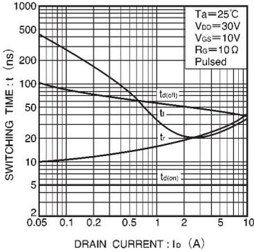
Fig.13 Switching characteristics
