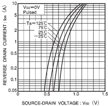
Fig.10 Reverse drain current vs. source-drain voltage (I)
