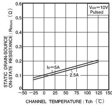
Fig.8 Static drain-source on-state resistance vs. channel temperature
