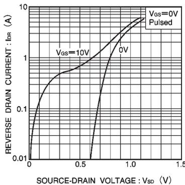
Fig.10 Reverse drain current vs. source-drain voltage ( II )
