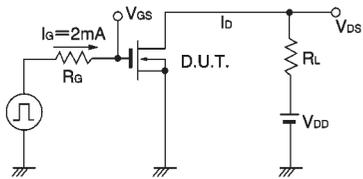
Fig.18 Gate charge time measurement circuit
