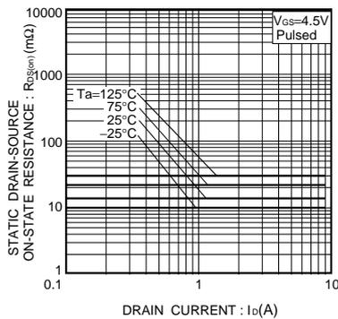
Fig.8 Static Drain-Source On-State Resistance vs. Drain Current (2)
