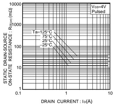
Fig.9 Static Drain-Source On-State Resistance vs. Drain Current (3)
