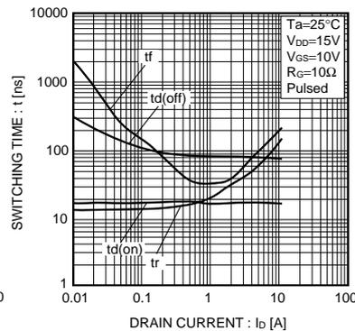
Fig.9 Switching Characteristics
