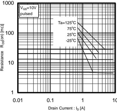
Fig.2 Static Drain-Source On-State Resistance vs. Drain Current (1)
