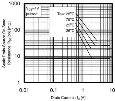
Fig.4 Static Drain-Source On-State Resistance vs. Drain Current (3)
