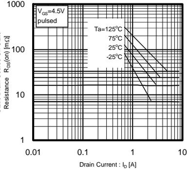
Fig.3 Static Drain-Source On-State Resistance vs. Drain Current (2)
