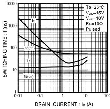
Fig.2 Switching Characteristics
