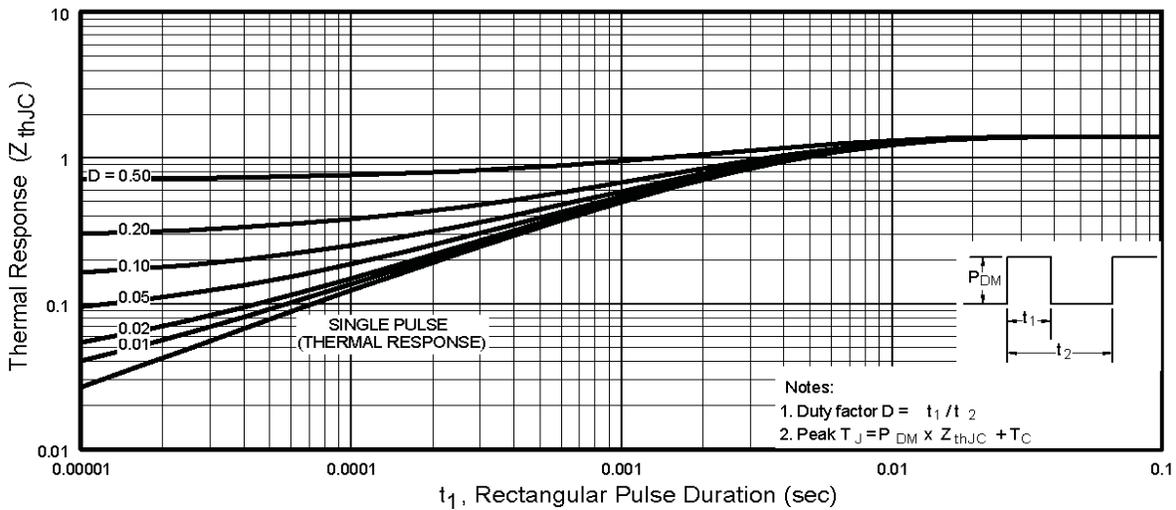
**Fig 11.** Maximum Effective Transient Thermal Impedance, Junction-to-Case
