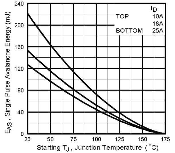
**Fig 12c. Maximum Avalanche Energy vs. Drain Current**
