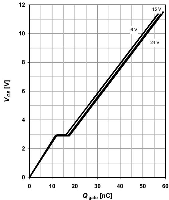
**16 Gate charge waveforms**
