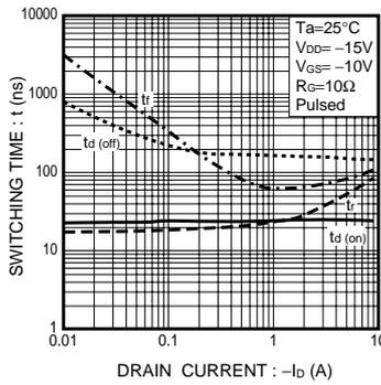
Fig.8 Switching Characteristics
