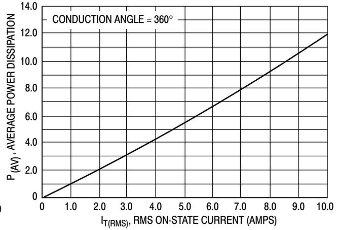
Figure 2. Power Dissipation
