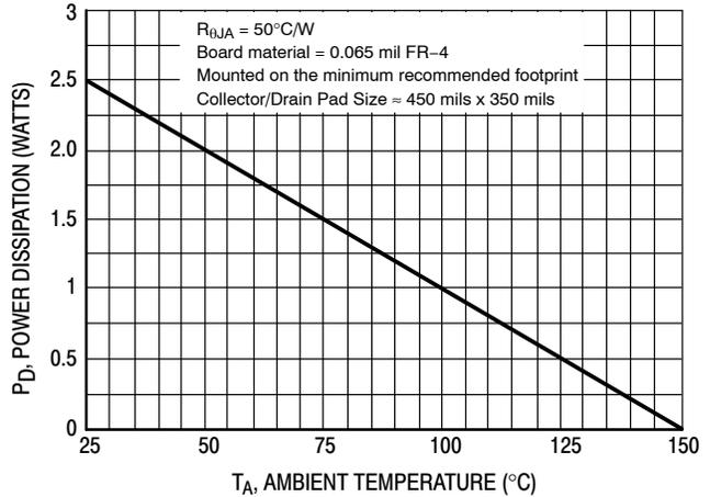
Figure 16. D<sup>2</sup>PAK Power Derating Curve
