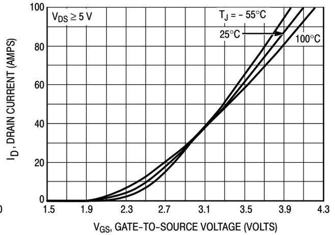
Figure 2. Transfer Characteristics
