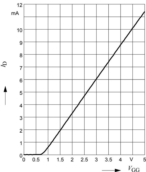
**Drain current  $I_D = f(V_{GG})$**
