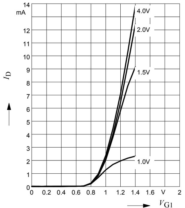
**Drain current  $I_D = f(V_{GG})$**
