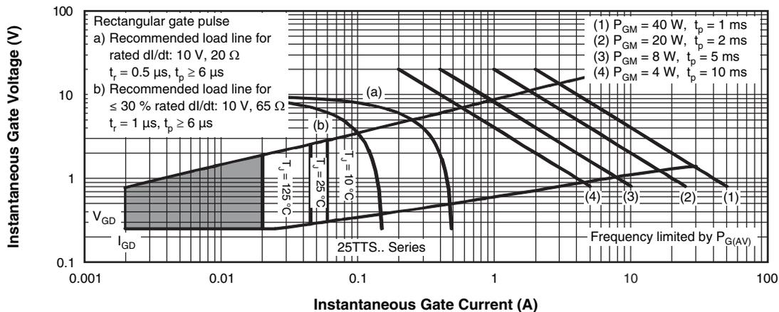
Fig. 8 - Gate Characteristics
