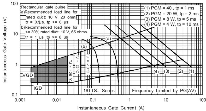
Fig. 9 - Gate Characteristics
