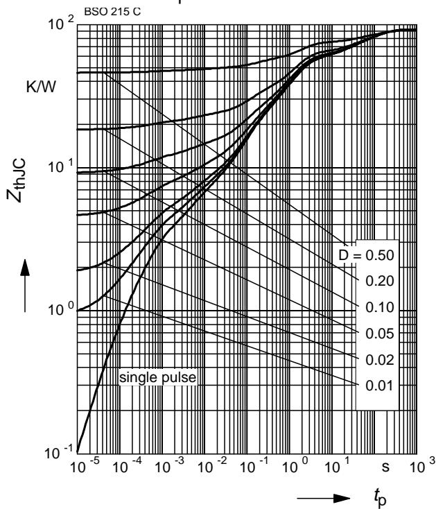
**Transient thermal impedance (P-Ch.)**
