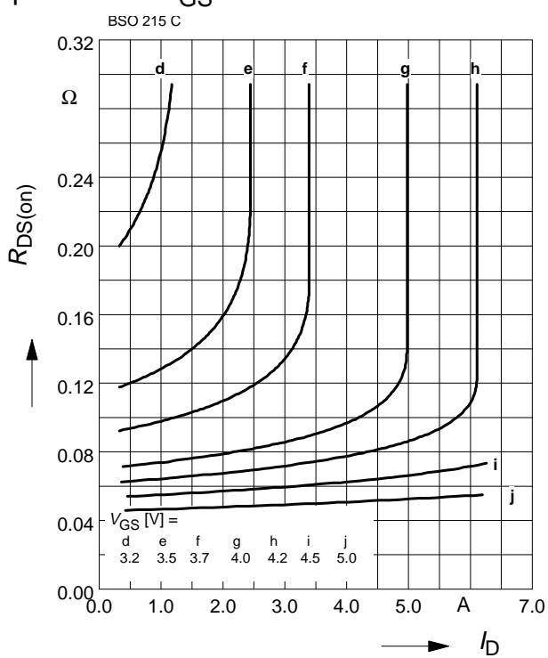
**Typ. drain-source-on-resistance (P-Ch.)**
