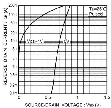
Fig.10 Reverse drain current vs. source-drain voltage ( II )
