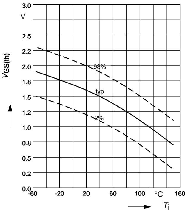
**Gate threshold voltage (P-Ch.)**
