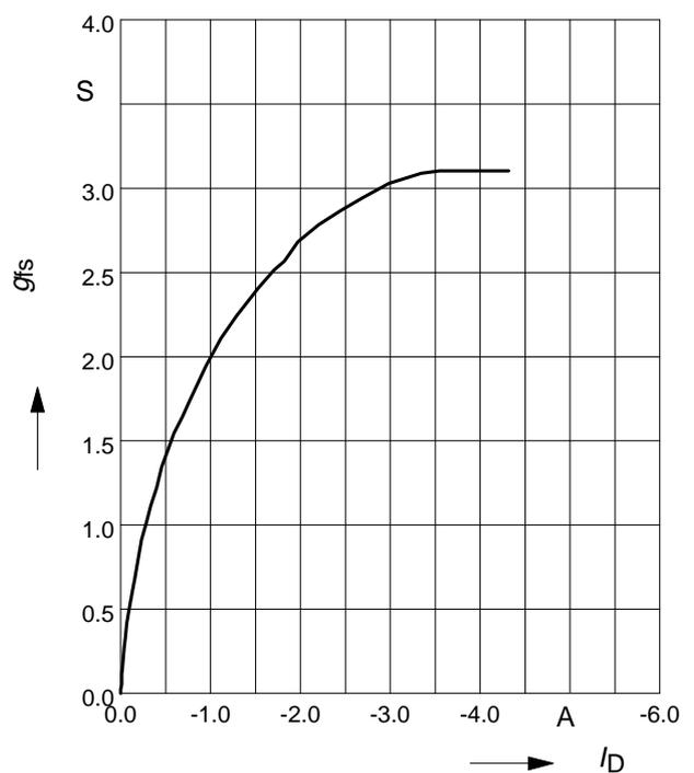
**Drain-source on-resistance (N-Ch.)**
