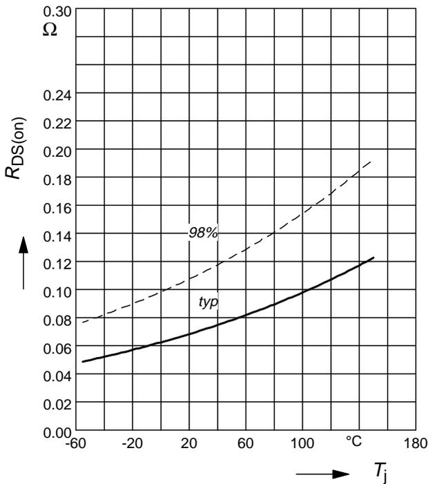
**Drain-source on-resistance (P-Ch.)**
