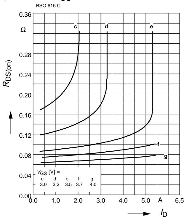
**Typ. drain-source-on-resistance (P-Ch.)**
