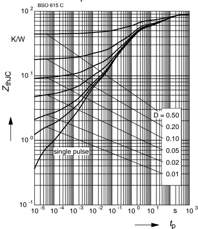
**Transient thermal impedance (P-Ch.)**
