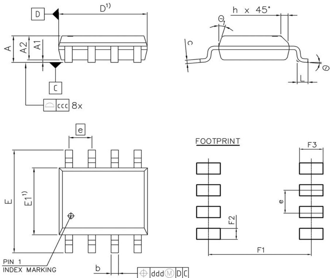
1) DOES NOT INCLUDE MOLD FLASH OR PROTRUSIONS.
