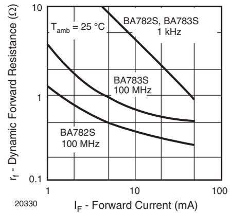
Fig. 2 - Dynamic Forward Resistance vs. Forward Current
