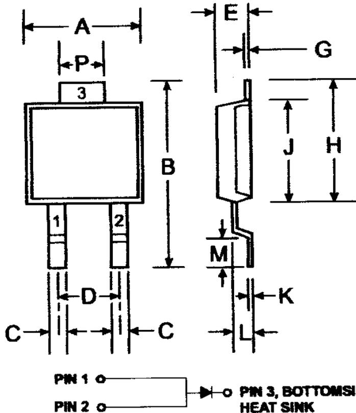
**Note:** Pins 1 & 2 must be electrically connected at the printed circuit board.
