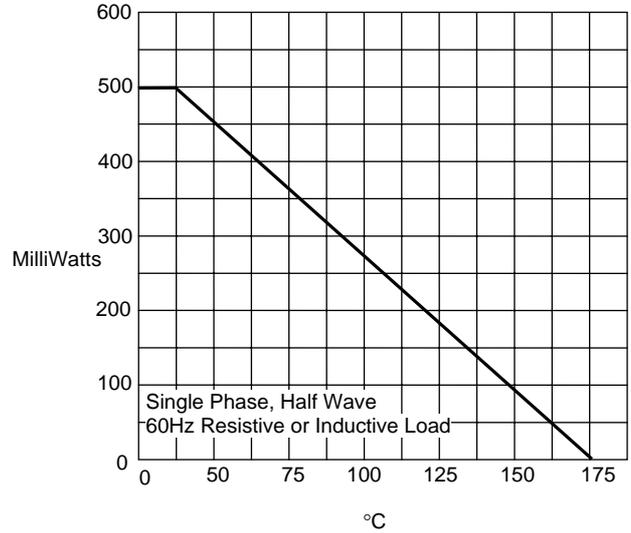
Admissible Power Dissipation - MilliWatts versus
