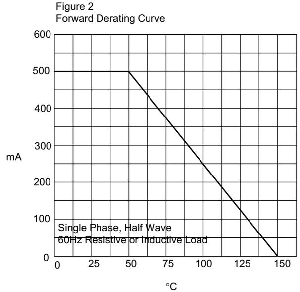
Average Forward Rectified Current - Amperes versus
