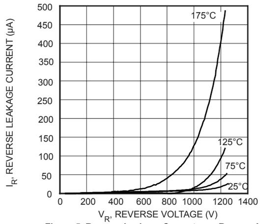
Figure 5. Reverse Leakage Currents vs. Reverse Voltage
