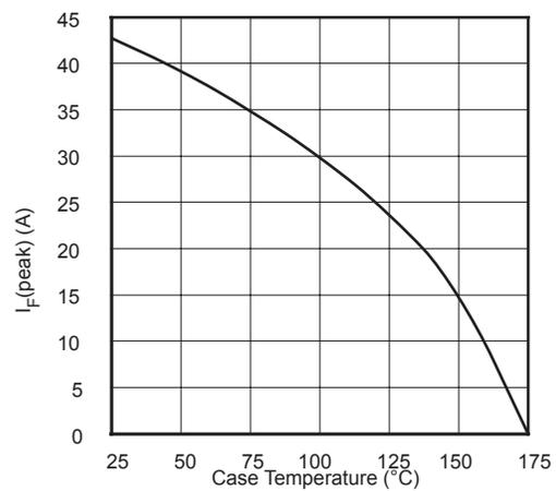
FIGURE 3, Maximum Forward Current vs. Case Temperature
