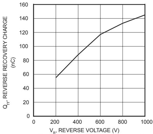
Figure 6. Reverse Recovery Charge vs. V<sub>R</sub>
