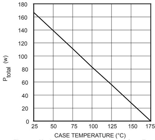
Figure 4. Maximum Power Dissipation vs. Case Temperature
