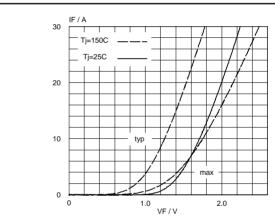
Fig.6. BY359X-1500S forward characteristic  $I_F = f(V_F)$ ; parameter  $T_i$
