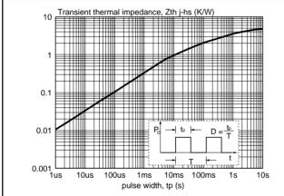
Fig.4. Transient thermal impedance  $Z_{th} = f(t_p)$
