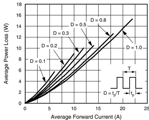
Figure 2. Forward Power Loss Characteristics Per Diode
