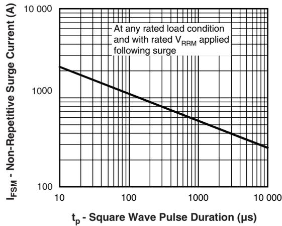
Fig. 7 - Maximum Non-Repetitive Surge Current (Per Leg)
