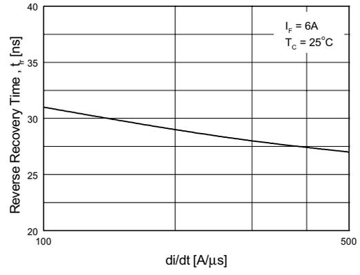
**Figure 4. Typical Reverse Recovery Time vs. di/dt**
