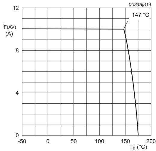
**Fig 3. Average forward current as a function of heatsink temperature; per diode; maximum values**
