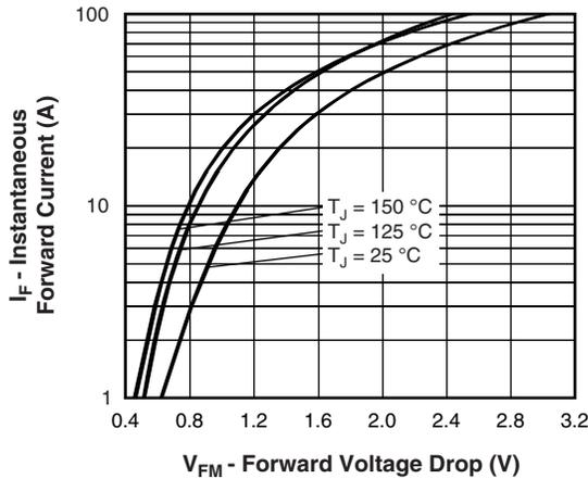
Fig. 1 - Maximum Forward Voltage Drop Characteristics (Per Leg)
