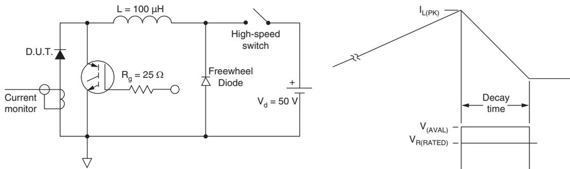
Fig. 11 - Avalanche Test Circuit and Waveforms
