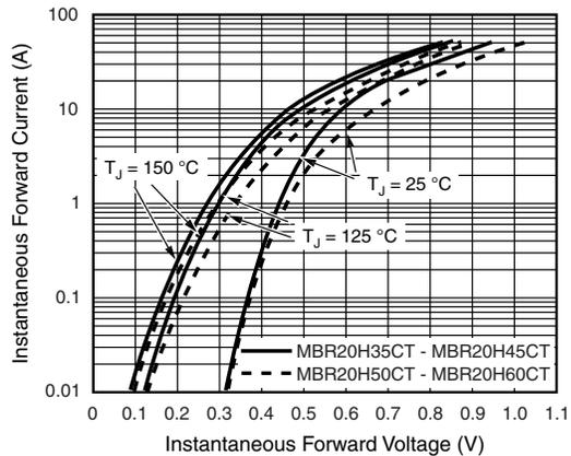
Figure 3. Typical Instantaneous Forward Characteristics Per Diode
