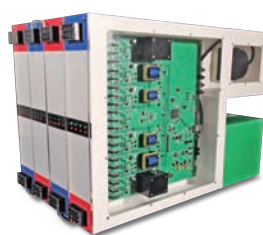
32kV rating switch modules (Voltage level can be adjusted depending on the number of modules connected in series.)
