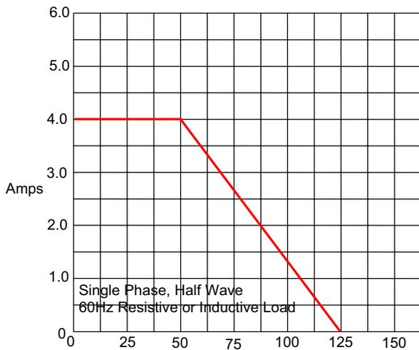
Average Forward Rectified Current - Amperes versus Case Temperature - °C
